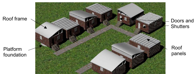
Fig. 1. Repurposing concepts for housing from 100-m long blade parts.
