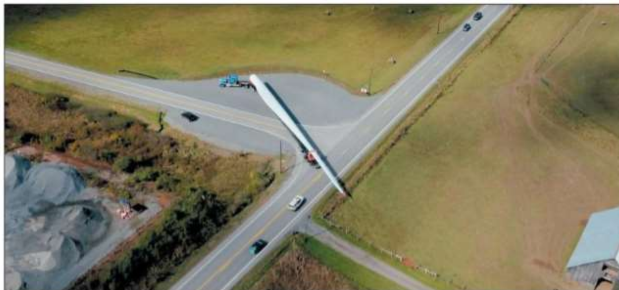
Greenville-based Logisticus manages the transport of turbine blades, some reaching almost 165 feet long, after the blades are retired from service. (Photo/Provided)
