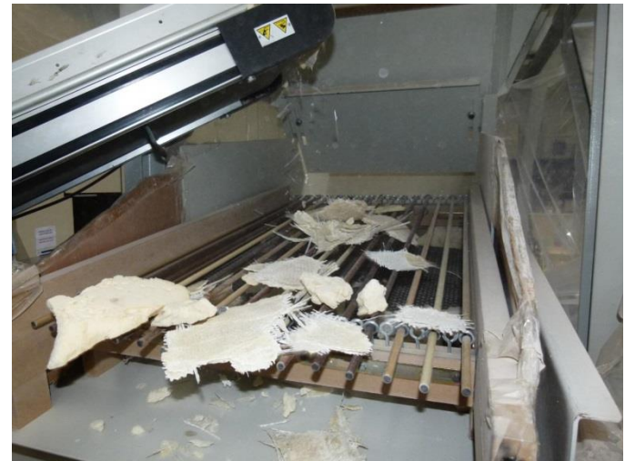
Cut GFRP composite waste Image: BRIO project Credit: Elhuyar Fundazioa
