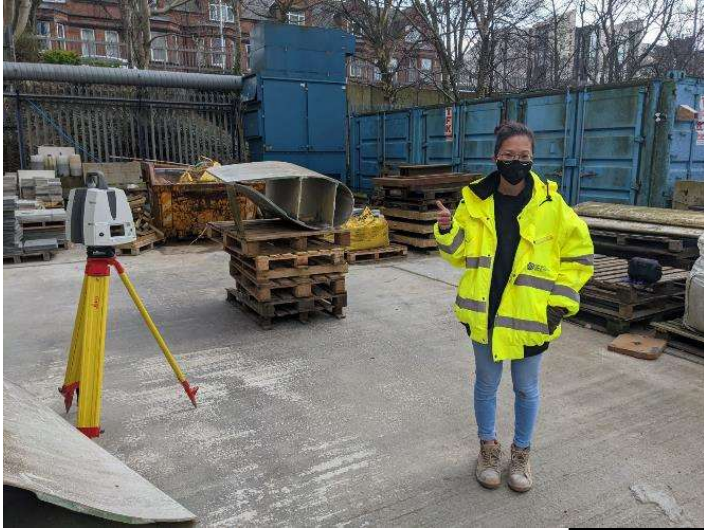
LiDAR scans of Vestas V52 (using Leica ScanStation P30/P40)
